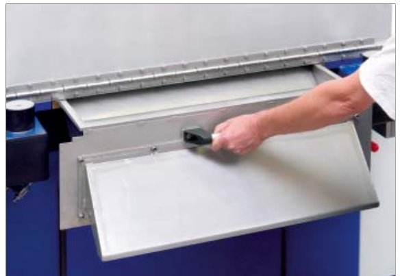
Discharge and cleaning of the strand outlet chute is much more convenient with a drawer system.
