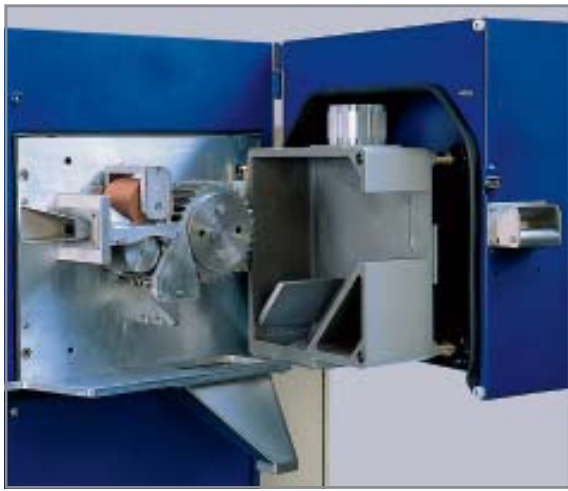
SGS 200-EL with opened pelletizer housing
