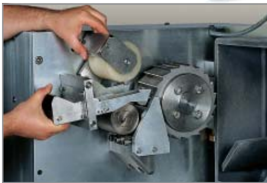
The infeed chute can be changed without using any tools
